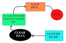
*Procedure of registration:* In this step firstly, the admin will create a database. In this diagram we refer admin with the master mode. The database created by admin consists of unique identification number, user name, password, mobile number, date of birth, photo, thumb image, address. The admin will load fingerprint of each individual with his/her personal information
